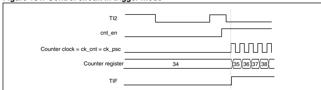
Figure 181. Control circuit in trigger mode
